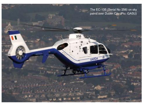
waypoints from the GPS. The EC-135 is powered by twin Turbomeca Arrius 2B2 engines which give a combined power output of 900KW.
