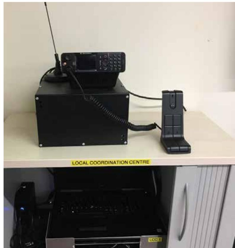
Figure 11. The TETRA base station installed in the Local Co-ordination Centre (LCC).
