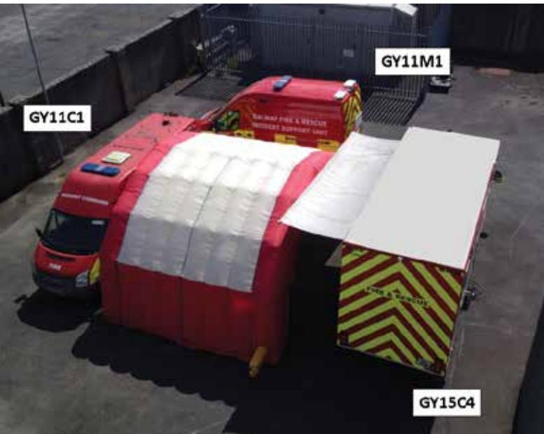
Figure 5. The layout of the Modular Command Centre, including an air-shelter.
